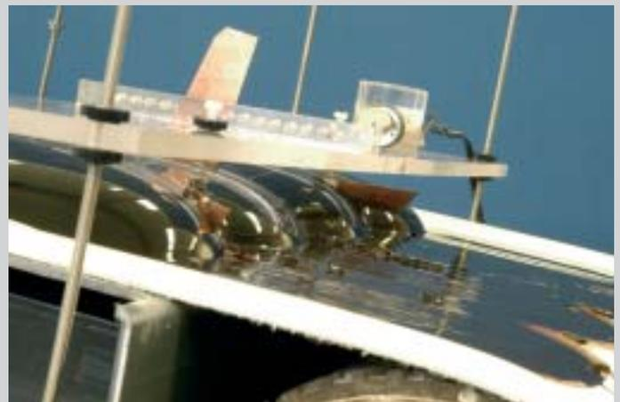
A separator vane inserted into the fluid down to 2 cm above the belt is used to separate the floating particles from those lying on the belt. The heavier particles move under the vane and drop off the end of the belt. The lighter particles float over the vane to hit a V-shaped ridge that carries them away to the side of the belt.
