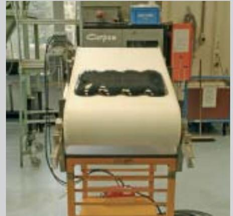
The 2 litre blob is held in place by a heavy permanent magnet located directly below the belt. The magnet consists of nine poles and weighs about 120 kilograms.
