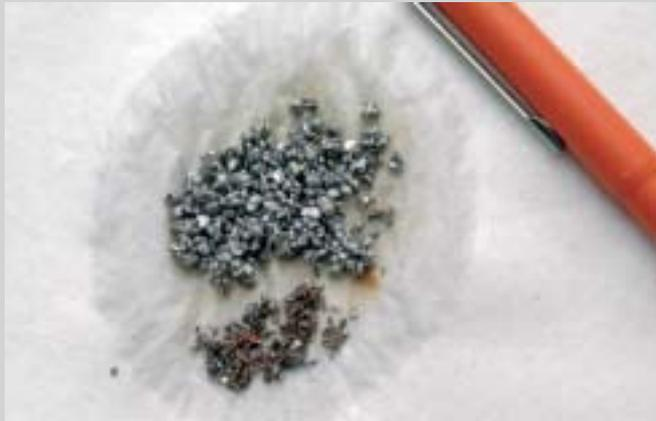
Separated particles of aluminium and copper.
