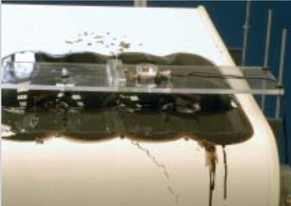
The metal particles are extracted in two flows, one in the centre, and one along the edge.
