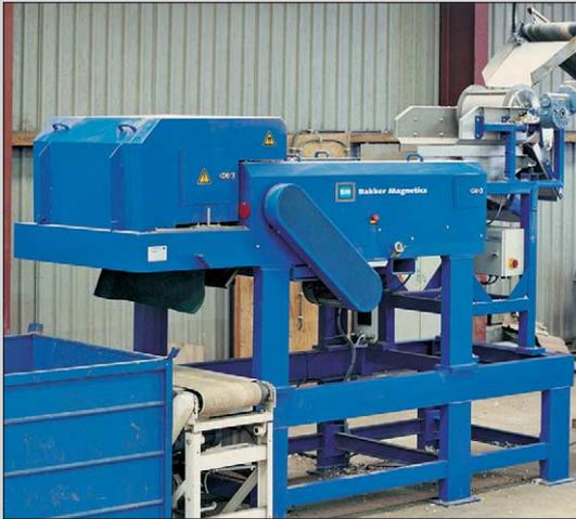
Eddy current separator used for separating aluminium from PET waste. It uses a rapidly changing magnetic field to eject the aluminium particles from the mixture.
