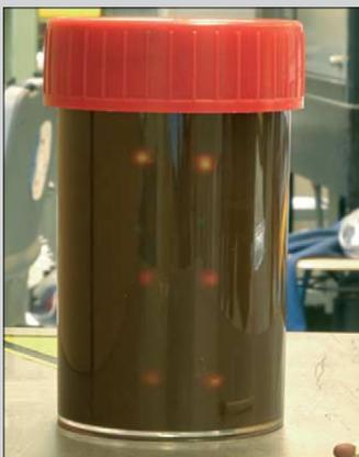
By making use of the decreasing effect of the magnetic field at higher level in the liquid, balls made of different types of plastics will float at different levels according to their specific gravity, with the heavy balls sitting lowest in the liquid, and the lightest ones at the top.
