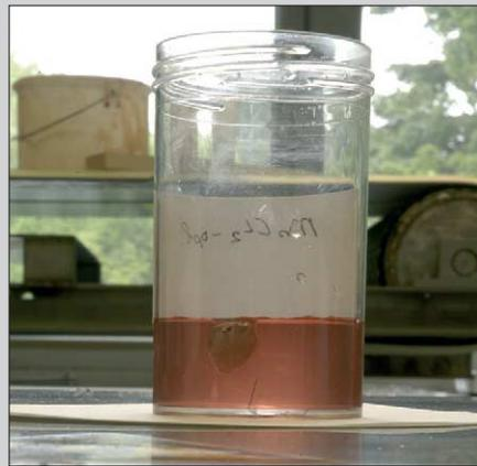
If a lump of magnesium (density approximately 1700 kg/m<sup>3</sup>) is dropped into a manganese chloride solution (density approximately 1400 kg/m<sup>3</sup>), it sinks to the bottom. If the container holding the solution and the metal is then placed on a magnet, the metal will rise in the solution (picture on the right) because of the increased density of the fluid.
