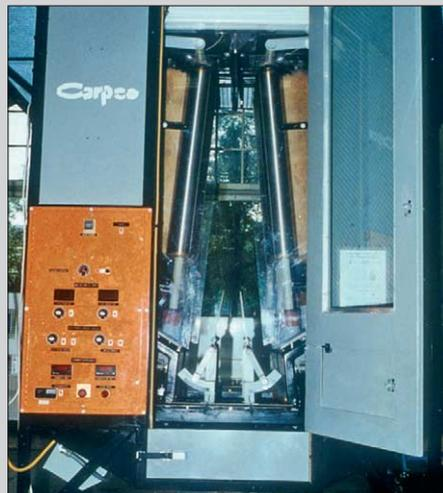
Electrostatic separator for removing PVC particles from shredded PET waste. Intensive stirring of the mixture imparts different electrostatic charges to the PET and PVC particles. The mixture is then dropped between the two vertical electrodes, across which a 60,000 volts electrostatic field is maintained. As they drop past the electrodes, the PET and PVC flows become separated.
