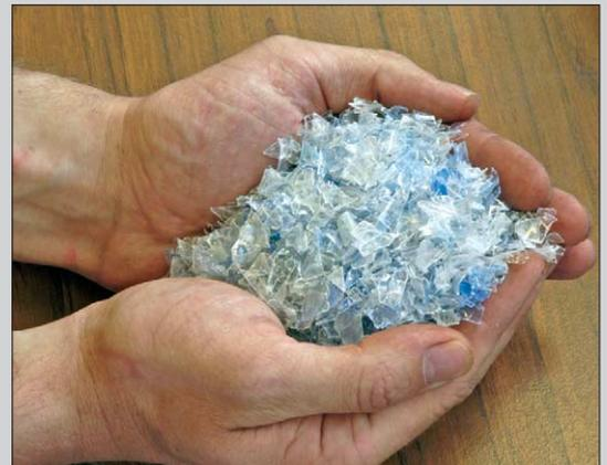
In order to process recycled PET bottles, they are shredded and any dirt and other unwanted materials such as bottle caps, labels, and whatever consumers have left behind, are removed.
